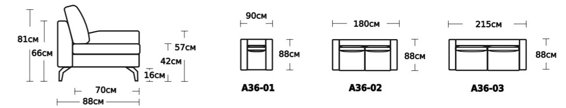
Complex solid frame - plywood, chipboard, zig-zag springs; Legs - chrome plated metal; Seats - polyurethane foam; Back cushions - silicone wadding; Warranty of construction - 2 years.
