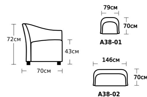
Complex solid frame - chip board, plywood; Legs - steamed beech; Seat - elastic belts, polyurethane foam; Back - polyurethane foam; Warranty of construction - 2 years.
