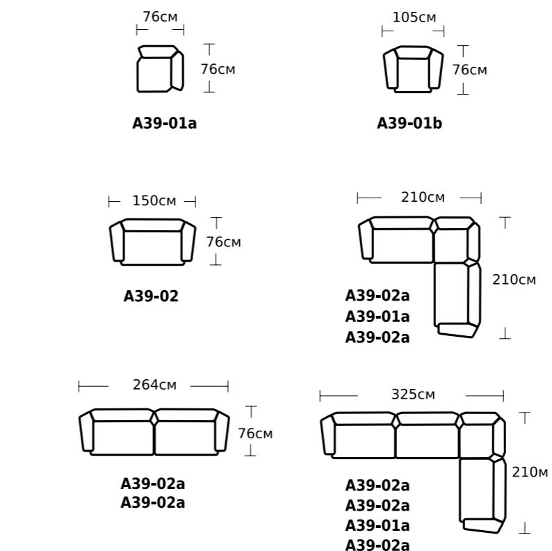
Complex solid frame - plywood; Legs - PVC coated steel; Seat - polyurethane foam; Back - polyurethane foam; Warranty of construction - 2 years.
